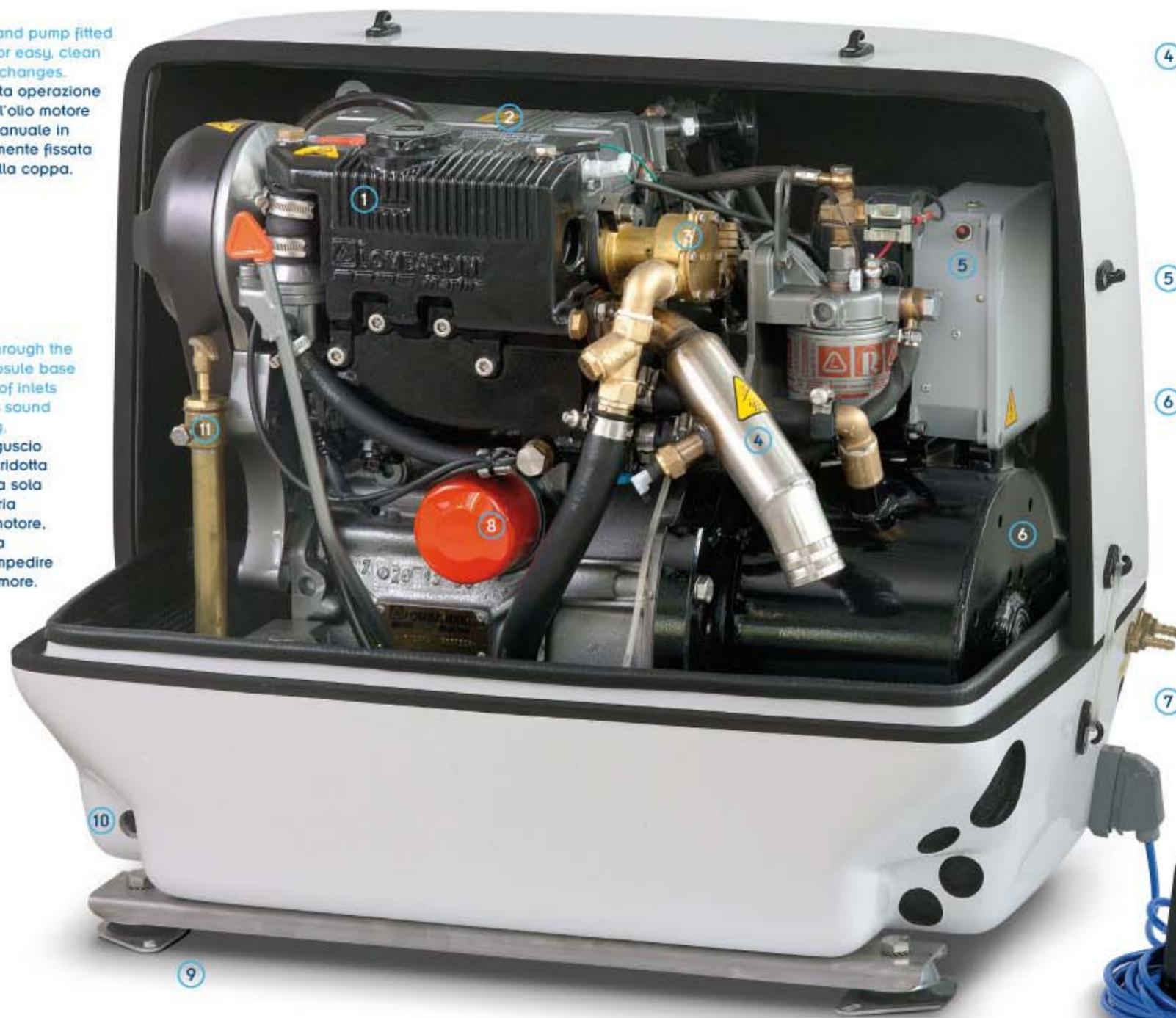
④ Exhaust and sprayed water manifold completely in stainless steel with high surface area cooling jacket. The cooled wet exhaust system ensures that no heat or vibration is transferred through the 45 mm. rubber hose.
